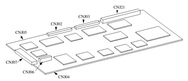
Figure 9-3. DTC PCBA
